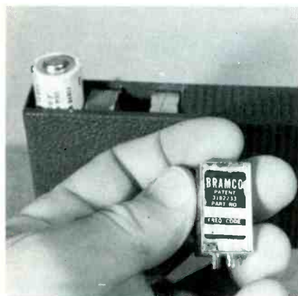
One of the reed assemblies is shown removed from the Code Call.
